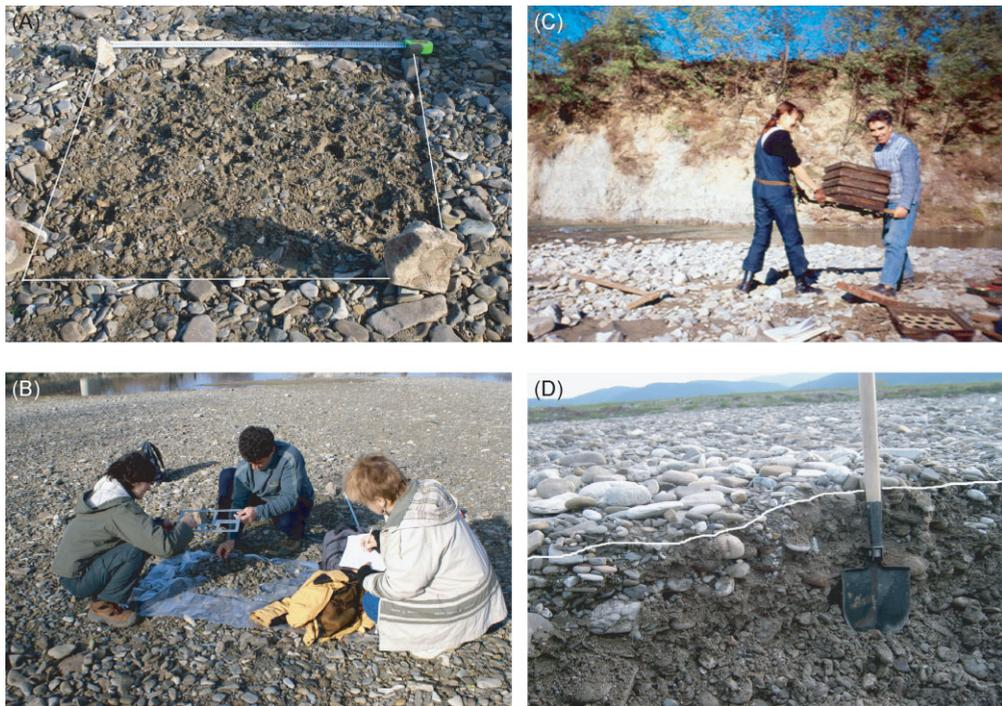
**Figure 3.** Illustration of the bed material sampling methods. (A) A sampling perimeter of one square meter; hand picking of surface material. (B) Surface material is collected on a plastic sheet. Each clast is measured using a gravel meter. (C) Use of hand sieving to separate the subsurface particles. (D) Vertical section in the Bistrita river-bed material. This figure is available in colour online at [www.interscience.wiley.com/journal/esp](http://www.interscience.wiley.com/journal/esp)
