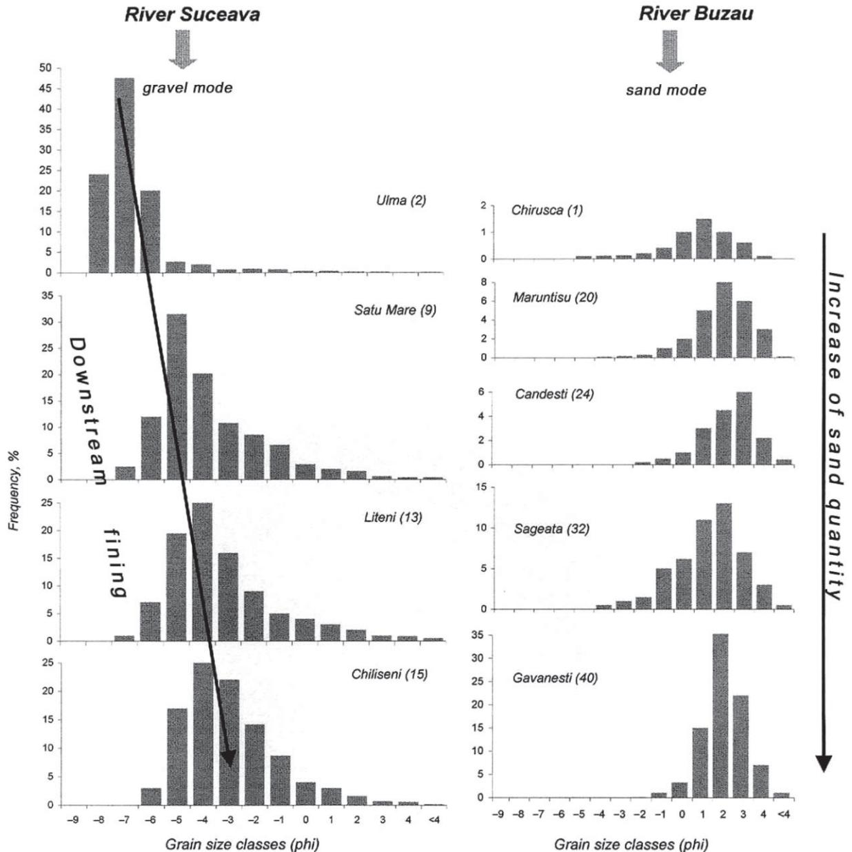
**Figure 11.** Grain size distributions of the gravel along the Suceava river (left). Grain size distributions of the sand along the Buzau river (right). Numbers indicate the position of sampling points below headwaters.
